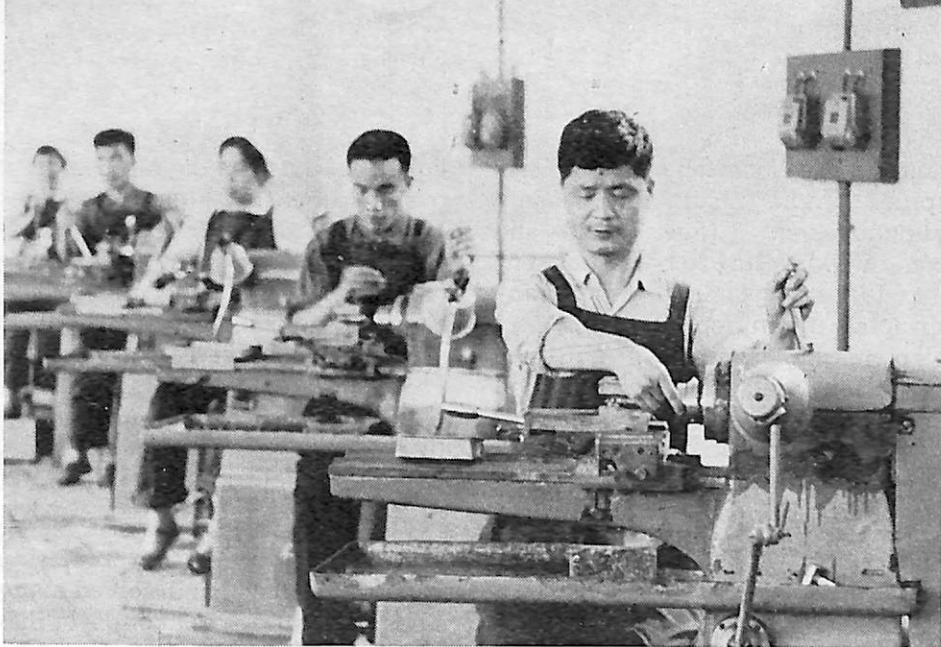
Chen Yu-chun (foreground) and other blind workers make brass nuts on special lathes.
